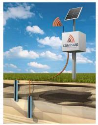
Installed system with multiple sensors, solar panel and GSM/GPRS transmission
