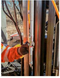
We have developed an adapter for push-in installation in soft clays. The adapter fits directly onto a 44 mm steel rod with R32 threading and protects the signal cable as it is pressed down. This method makes installation without permanent pipes in the ground possible and is cost and time-efficient.
