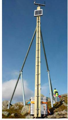
Installed systems with weather station. The logger is placed either in a cabinet on the mounting post or in a case on the ground.
